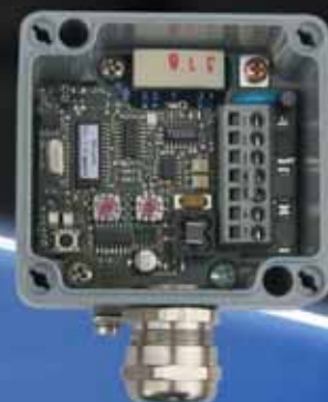
Inclination angle transmitter
