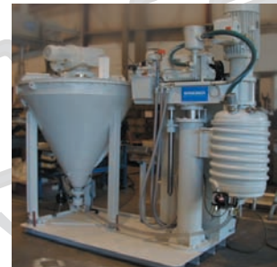
Vakuumdissolver (Co. Grieser) Mixing of special paints
