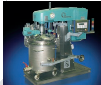
Kreis-Dissolver (Co. Niemann) Dissolving of high viscosity pastes
